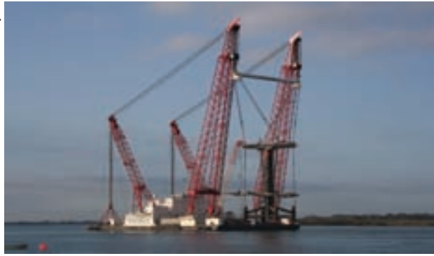
SeaGen being transported by crane barge Rambiz
